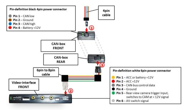
Connect black female 4pin Micro-Fit connector of the 4pin cable to the male 4pin Micro-Fit connector of the CAN-box.
