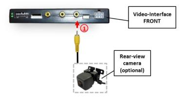
1 Connect the video-RCA of the after-market rear-view camera to the female RCA port of the video-interface which is labeled as CAM.
